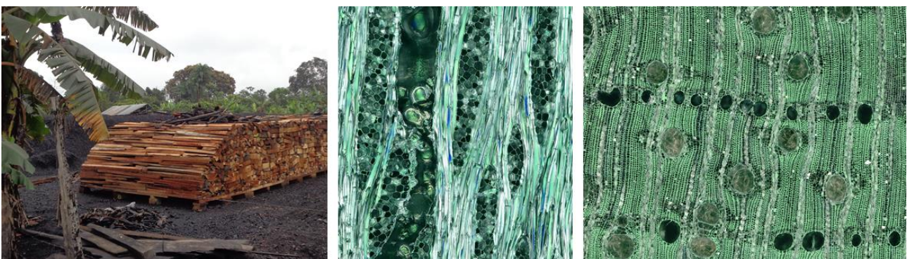
Left: Charcoal Miller with residual wood in Peru, Middle: Tangential section of Teak charcoal, Right: Transverse section of "Copaifera-Type" charcoal.
